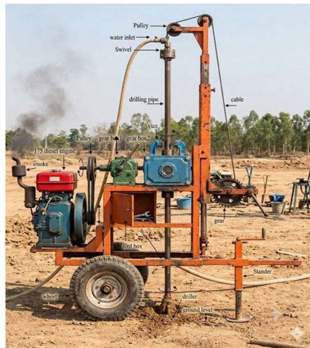
Figure 2. Rotary drilling machine after construction
